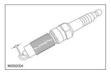
2. NOTICE: Only use hand tools when removing or installing the spark plugs or damage can occur to the cylinder head or spark plug.
